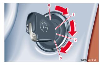
0 The electronic key can be withdrawn in this position only. The steering is locked when the electronic key is removed from the steering lock. If necessary, move steering wheel slightly to allow the locking mechanism to engage. The electronic key can only be removed with the selector lever in position "P". After removing the electronic key or with the electronic key in steering lock position 0, the selector lever is locked in position "P".
